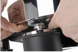
Gently lift the platter edge exposing the motor pulley.
