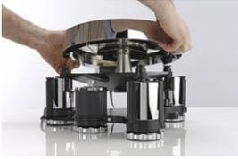
Carefully fit the platter to the bearing, making sure the location of the fitting pin is between the motor and the front left suspension housing.
