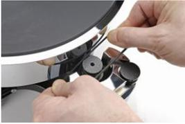
Fit the lateral suspension O-rings to each suspension tower.
