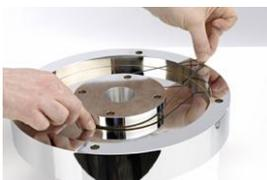
Always make sure you have clean hands when handling the drive belts and before fitting the belt it is a good practice to clean the platter drive hub and motor drive pulley. Isopropyl alcohol cleaner would be suitable.
