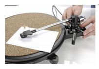
Sliding the arm back and forth is simply done by moving the carriage. Once this is completed, tighten the fixing bolts down and make final check of the VTA, making any adjustments as required.
