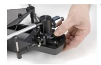
Fit the whole assembly to the subchassis using the M3 x 20 bolts, M3 washers and M3 nuts supplied. Do not tighten down and keep loose. Fit the arm wand making sure the arm connecting cable is not caught. Fit into the receiving socket and check movement is not restricted. If it is you may need to reposition the sockets orientation.
