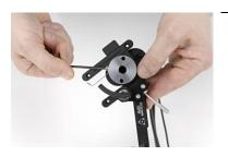
Fit the bias hanger carefully with the same bolt, facing forward, initially parallel to the siding bar and the base of the bias hanger parallel the to sliding carriage.
