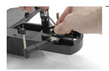
You may find some cartridges that are very high, such as Dynavector that spacers will not be enough. An additional higher cue casing is included which can be fitted to give you the correct height. The cue mechanism will need transferring from one to the other and you should either consult your dealer or contact us if you have difficulty with this.
