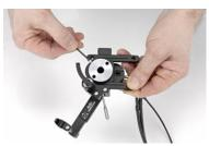
Remove the bias hanger-retaining bolt.
