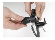
Now fit the retaining nut but do not over tighten. It may be necessary to rotate the mounting collar later. **DO NOT USE THE NAIM NUT SUPPLIED**
