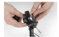
Making sure the sliding bars are in place, replace the plastics transit bolt with the Naim mounting collar.
