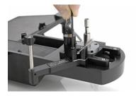
Refit the cue mechanism with the longer bolts supplied. Replace the arm and make any final adjustments altering the height of the arm cue bar as required.
