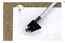
Using the protractor supplied adjust the overhang. The protractor has been specifically designed for the Naim ARO. It should make it easy to obtain the correct alignment by placing the stylus on the centre mark and then 'sliding' the base back and forth until the cartridge is correctly aligned.
