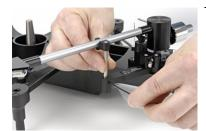
Adjust the arm holder to the correct height using the locking screw. Now remove the wand the fit your cartridge. Set the tracking weight using the counterweight and suitable scales. With the bearing, platter, record and clamp fitted check the VTA of the arm. If required remove the wand and adjust the height of the pillar/bearing.
