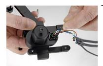
Attach the arm cable to the underside of the Naim Slide assembly, using the  $4 \times M2$  bolts supplied.
