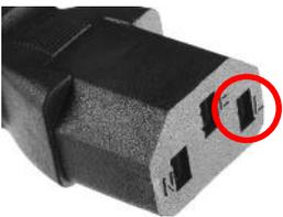
For users who have to use two-pin mains sockets, please note that on a standard IEC mains female plug, the right hand pin (see image) is the 'Live' pin—always make sure this is connected to the live pin on the wall socket. Failure to do so will mean that the neutral feed will pass through the mains switch rather than the live feed, which is less safe and should be avoided.
